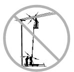
Keep away from the machine if it contacts energized power lines or becomes electrically charged. Personnel on the ground or in the platform must not touch or operate the machine until energized power lines are shut off.
