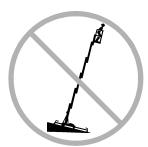
Do not raise the platform unless the machine is on a firm, level surface. The machine is intended for use on level surfaces only.
