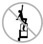
Do not exit the platform while raised. If a power failure occurs, have ground personnel activate the manual lowering valve.
