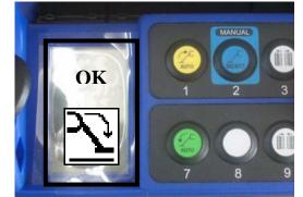
It is also possible to operate the outriggers manually, by pressing button no. 2 (blue one) and following the instructions on the display (not recommended procedure).
