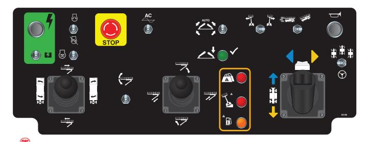
**IMPORTANT**—Before moving, check that the route of travel to be taken is clear of persons, obstructions, debris, holes, and drop offs, and is capable of supporting the machine.
