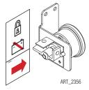
Check Battery Disconnect Switch outside the front end of the Engine Module.
