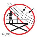
DO NOT work in close proximity to, or in contact with, energized power lines and electrical equipment. This machine is not insulated and WILL NOT protect the operator from injury or the machine from damage.
