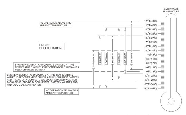
Figure 7-4. Engine Operating Temperature Specifications - Caterpillar - Sheet 1 of 2
