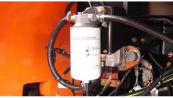
Lube Point(s) - Replaceable Element Interval - Drain water daily; Change every year or 500 hours of operation
