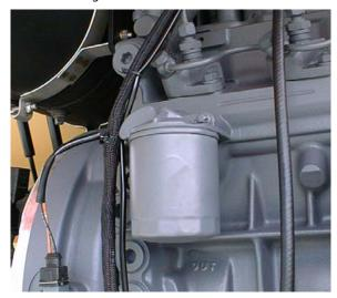
Lube Point(s) - Fill Cap/Spin-on Element Capacity - 11 Quarts (10.5 L) w/Filter Lube - FO
