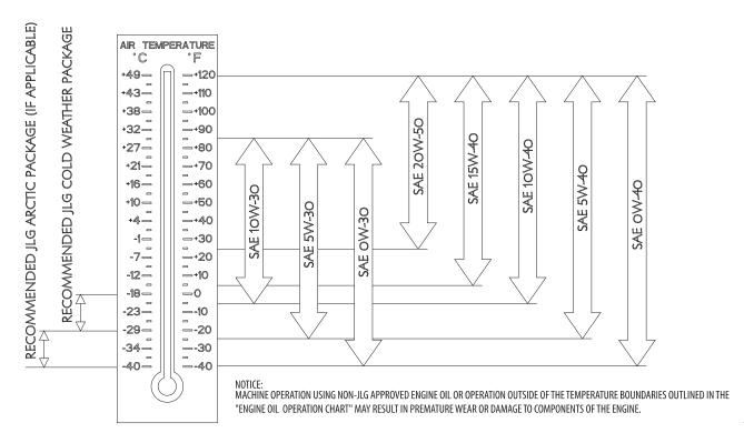
**Figure 7-1. Engine Operating Temperature Specifications**
