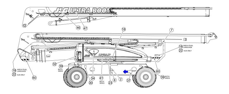
Figure 4-10. Decal Location Sheet 1 of 5
