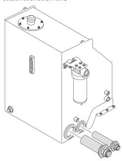
Lube Point(s) - 2 Interval - Every 2 years or 1200 hours of operation. Remove and clean at time of hydraulic oil change.
