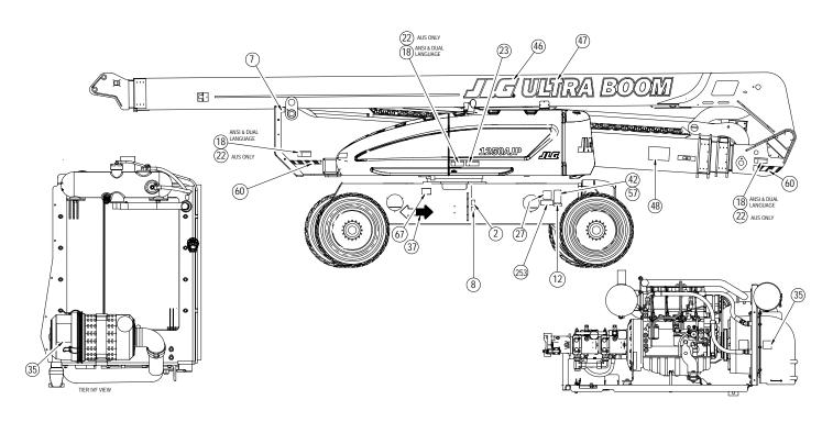
Figure 4-13. Decal Location Sheet 4 of 5
