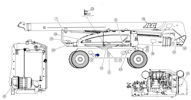
Figure 4-18. Decal Location - S/N 0300141446 to Present - CE Only - Sheet 4 of 5
