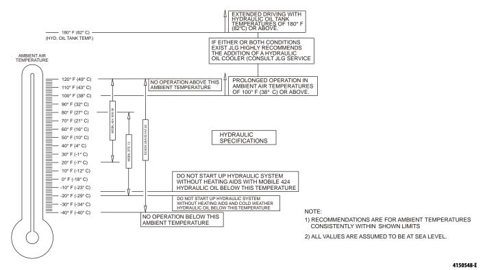
Figure 7-5. Engine Operating Temperature Specifications - Caterpillar - Sheet 2 of 2
