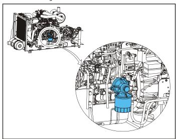
Lube Point(s) - Fill Cap/Spin-on Element (element can be accessed from below engine tray)
