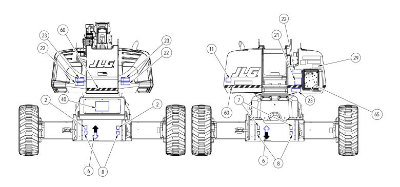
Figure 4-19. Decal Location - S/N 0300141446 to Present - CE Only - Sheet 5 of 5
