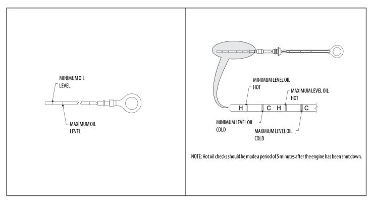
Figure 7-10. Deutz 2011 Engine Dipstick
