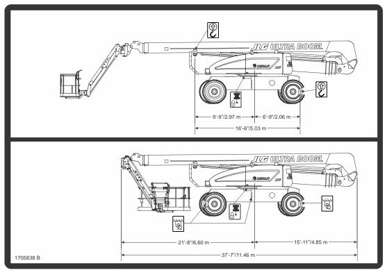
Figure 4-9. Lifting and Tie Down Chart
