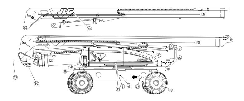
Figure 4-15. Decal Location - S/N 0300141446 to Present - CE Only - Sheet 1 of 5
