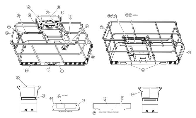
Figure 4-12. Decal Location Sheet 3 of 5
