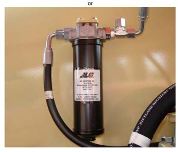
Lube Point(s) - Replaceable Element Interval - Change after first 50 hours and every 300 hours thereafter or as indicated by condition indicator (if equipped)
