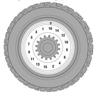
The tightening of the nuts should be done in stages. Following the recommended sequence, tighten nuts per wheel torque chart.
