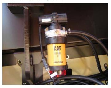
Lube Point(s) - Replaceable Element Interval - Drain water daily; Replace element every year or 600 hours of operation
