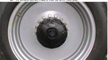
Lube Point(s) - Level/Fill Plug Capacity - 0.5 liters (1/2 full)
