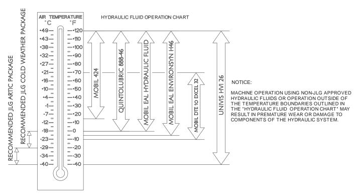
Figure 7-2. Hydraulic Oil Operation Chart - Sheet 1 of 2
