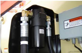
Lube Point(s) - Replaceable Element Interval - Change after first 50 hours and every 300 hours thereafter
