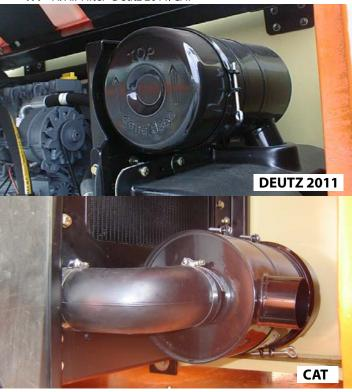
Lube Point(s) - Replaceable Element Interval - Every 6 months or 300 hours of operation or as indicated by the condition indicator
