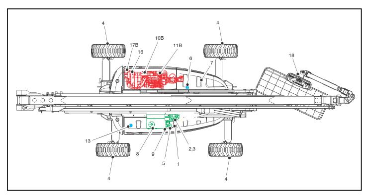
Figure 7-7. Operator Maintenance and Lubrication Diagram - Deutz 2.9 Engine
