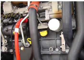
Lube Point(s) - Fill Cap/Spin-on Element
