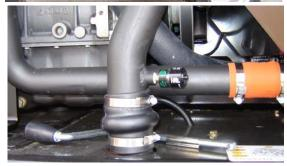
Lube Point(s) - Replaceable Element Interval - Every 6 months or 300 hours of operation or as indicated by the condition indicator Comments - Check Dust Valve daily
