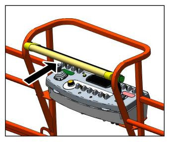
**NOTE:** If the machine is equipped with both SkyGuard and Soft Touch, functions will not reverse, only stop.
